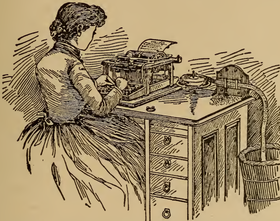
Fig. 4. ROGERS' TYPEWRITER PREPARING TAPE.
